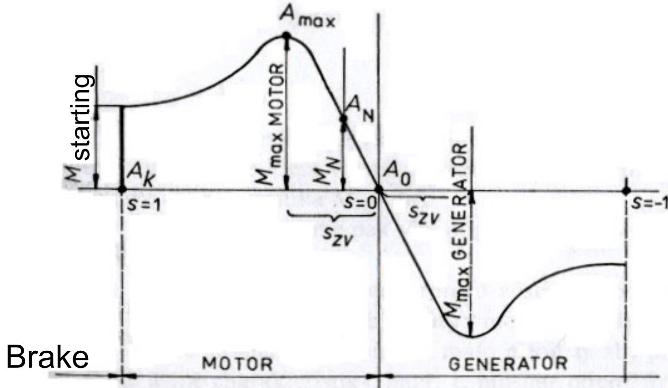
torque overload capacity
